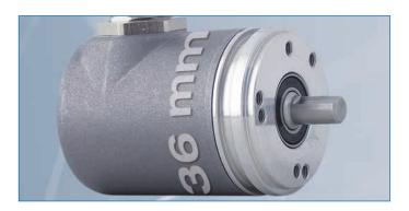
The new series of WDGP incremental encoders offer the customer a significantly high resolution of up to 16,384 ppr in a very compact design from 36 mm. This means that highly precise measurements can be realised in the smallest installation space. The series can be supplied with any number of pulses from 1 to 16,384 ppr and a zero pulse. The zero pulse can be freely set. The electronics delivers in HTL or TTL with a frequency of up to 1 MHz to the ABN signals also the inverted ones.
